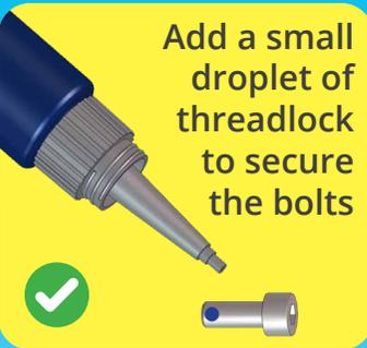
Add a small droplet of threadlock to secure the bolts
