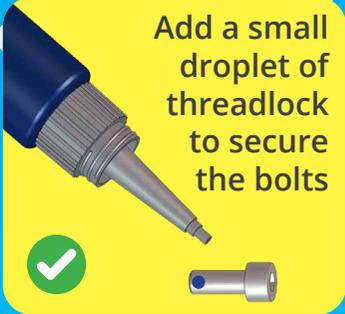
Add a small droplet of threadlock to secure the bolts
