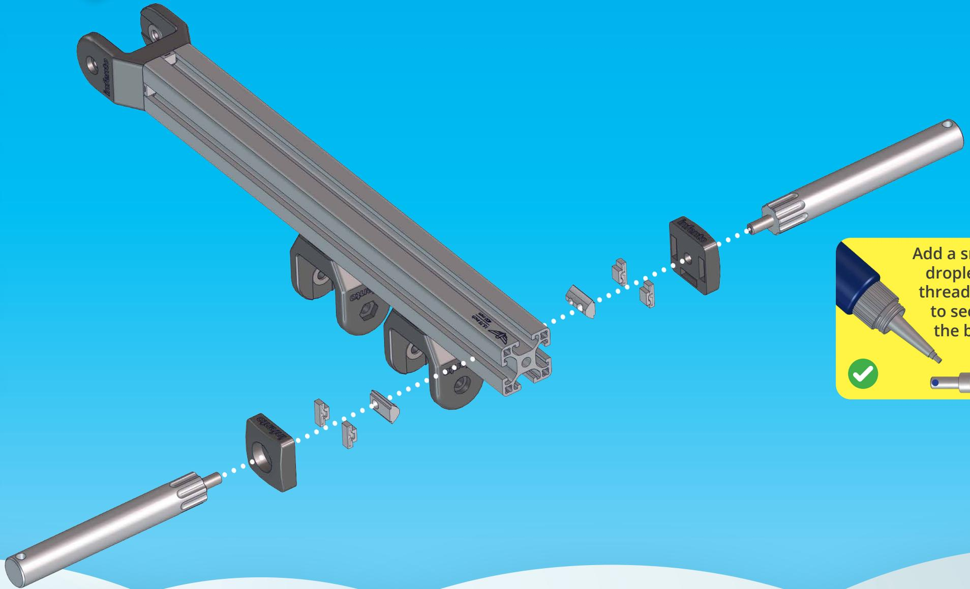
Add a small droplet of threadlock to secure the bolts
